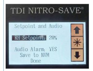
NOTE: The high humidity setpoint is factory programmed to 20%RH, which represents general electronics requirements. For more critical humidity control, reduce the setpoint and for less critical humidity control, increase the setpoint.
