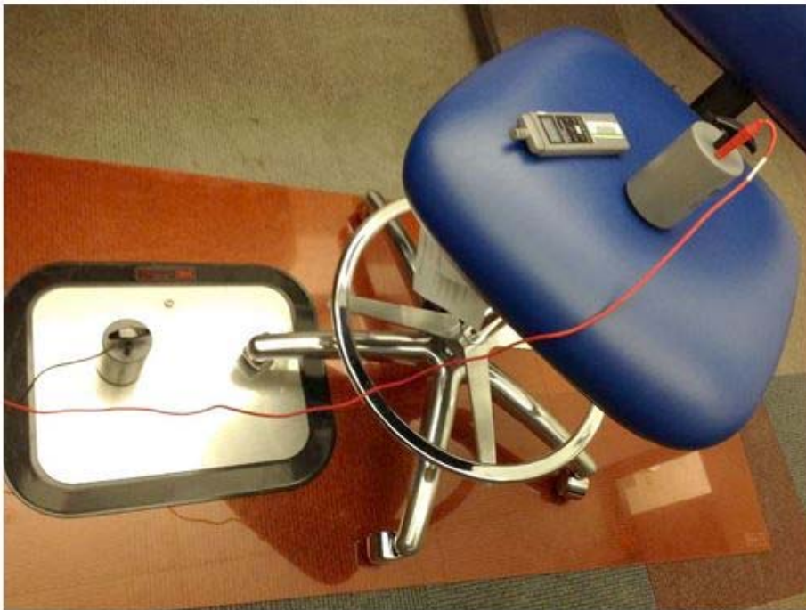
Figure 1 - Setup for 1 Wheel Measurement; Other 4 Wheels on Insulative Support Surface
